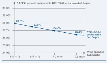
Calculation of AEP based on air density of 1.225 kg/m³, wind shear of 0.2 and Weibull shape parameter of k = 2.0
